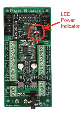
The lights kits should work just like before you wire in the battery connections to the Sound Board. Verify that the Power Switch does turn on and off power to the sound board (look at the power indicator LED) and all of the light boards. Also verify that the lights kits are operating properly before you go to the next step.
