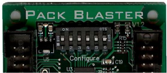
The switches are defined to be able to correct for different types of switches and switch connections (#1, #2 and #4), select which of 4 pack configuration will be used when the board is powered on (#3 and #5), and whether you want the pack to Hum when powered up and idling or not (#6).
