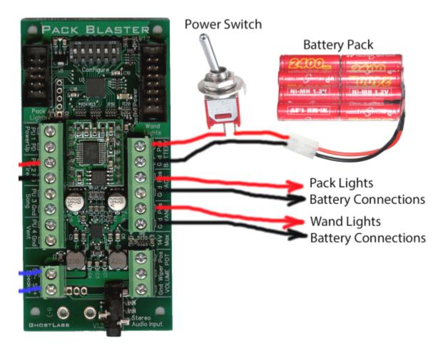
A 9V to 14V battery pack is used to power this board and also the pack and wand light kits if you have those. The battery is connected in parallel to all of these systems and to simplify your wiring the sound board has provided additional screw terminal connections to distribute the battery voltage to the other boards.
