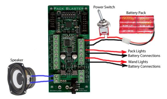
To make sure the sound board does not try to output any sounds, set all six of the Configuration Dip Switches to the OFF position (all switches toggled towards the bottom of the board):
