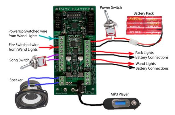
Since we are sharing the battery, only the live or switched side wire from the shared switches needs to be brought back to the sound board.
