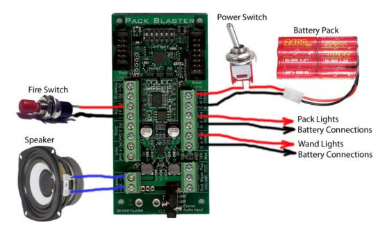
The Fire switch connections are labeled "PU" and "PD". One connection is made from each of these to one side of the switch. The order is not important and if the wire connections are swapped, the operation will still be the same.
