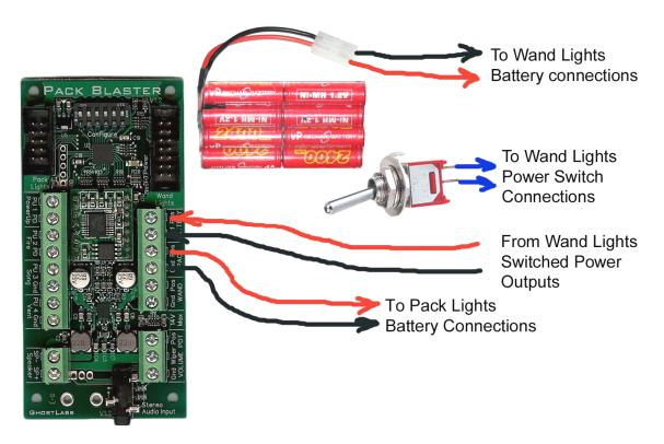
All three of the Sound Board's battery connections are just tied together and are used to help you simplify your wiring: No splicing wires together, just use the screw terminals on the sound board.
